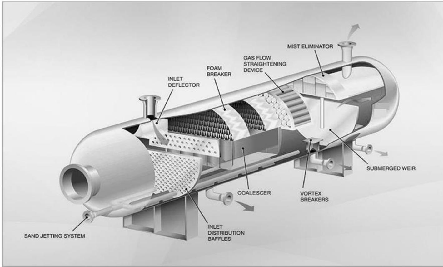
Figure-1: Internal Arrangement of Three Phase Crude Oil Separator
