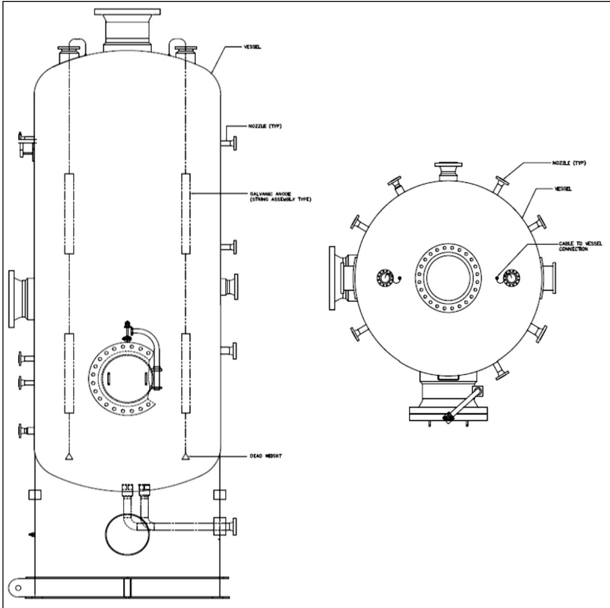
Figure-4: CP System for Vessel Internal with String Assembled Galvanic Anodes
