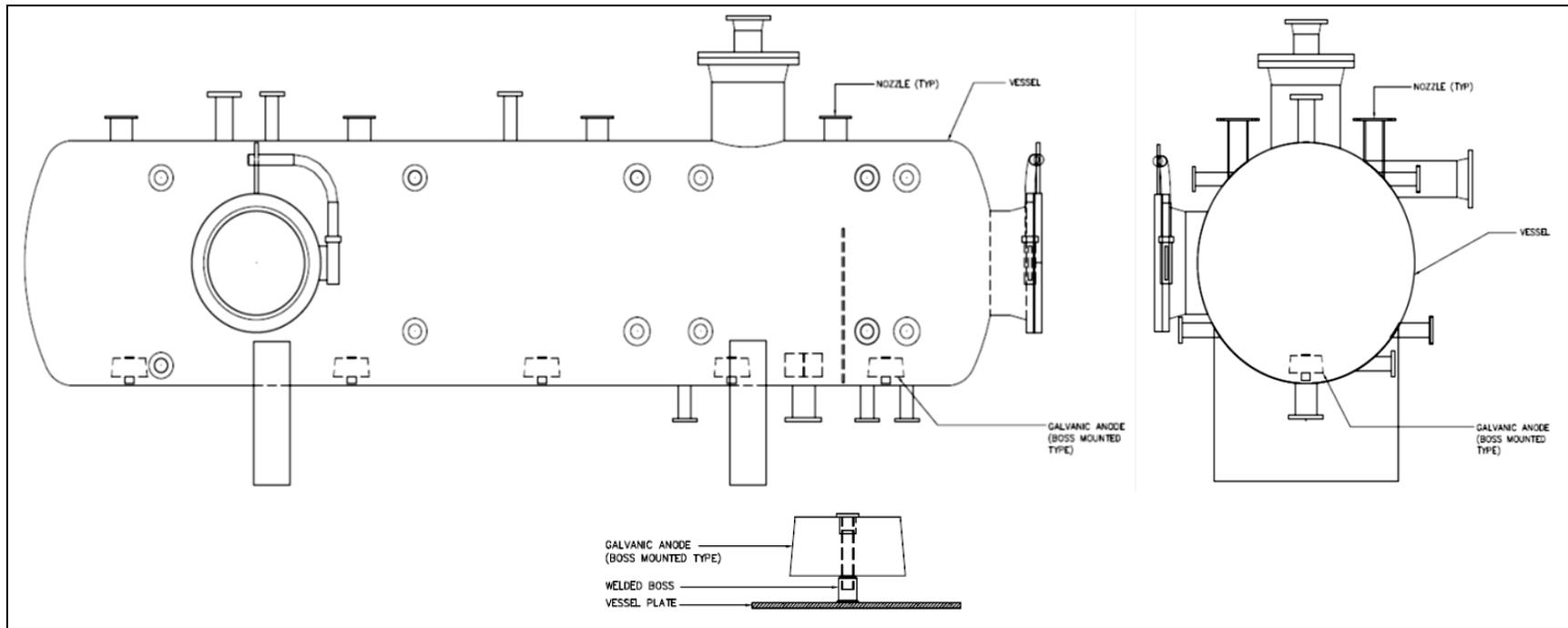
Figure-2: CP System for Vessel Internal with Boss Mounted Galvanic Anodes
