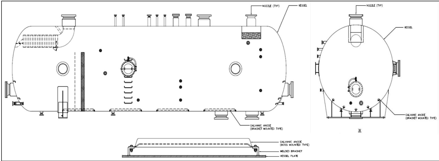
Figure-3: CP System for Vessel Internal with Bracket Mounted Galvanic Anodes
