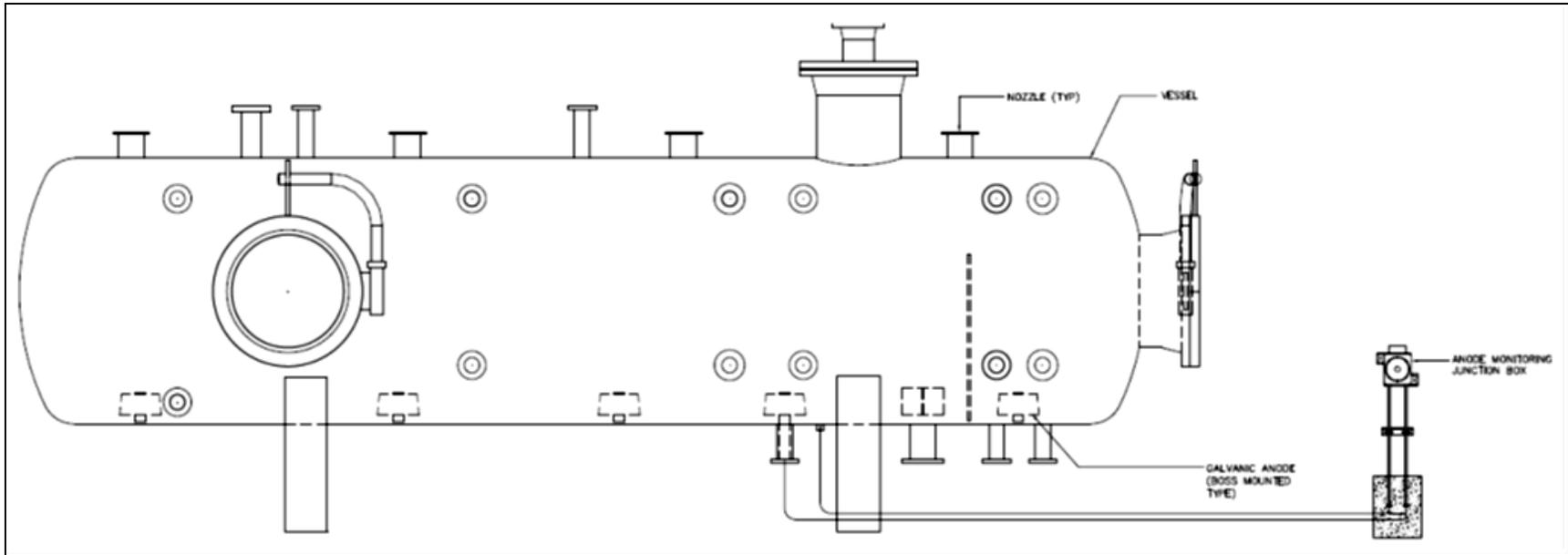
Figure-5: CP System for Vessel Internal with Anode Monitoring System
